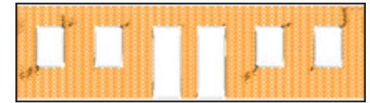
b) Moderate Damage Threshold (DT2) (maximum crack width - 5 mm).
