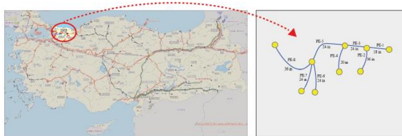
a) Turkish regional map and buried gas pipelines network b) High-pressure gas network of Düzce – Gebze regions as a test-bed scenario
