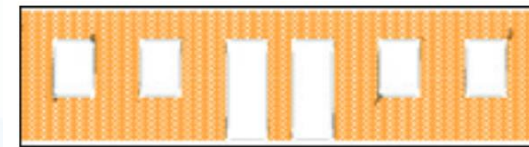
a) Slight Damage Threshold (DT1) (maximum crack width - 1 mm).
