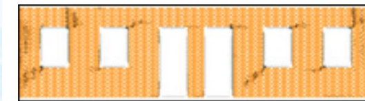
c) Extensive Damage Threshold (DT3) (maximum crack width - 10 mm).
