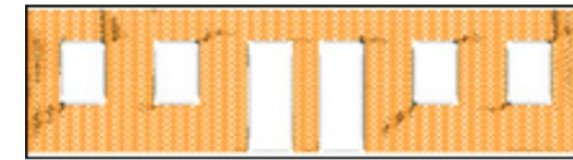
c) Extensive Damage Threshold (DT3) (maximum crack width - 10 mm).
