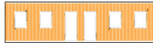
a) Slight Damage Threshold (DT1) (maximum crack width - 1 mm).
