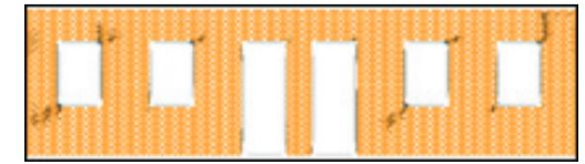
b) Moderate Damage Threshold (DT2) (maximum crack width - 5 mm).
